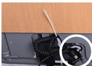
Remove the split pin and one of the washers. Locate the drilled hole in the platform. Insert the cable guide so that it protrudes through the other side of the frame. Replace the washer and split pin.
