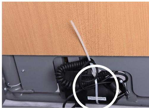
Pass the lift height adjustment motor cables under the platform and connect to the yellow ports on the control box
