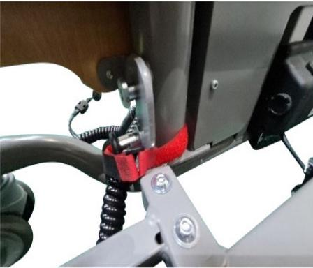
Lay the coiled cable over the crossbeam from the head or foot end as shown in the picture.
