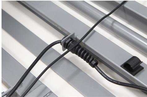
Fix the power cable to the chassis using the bracket at the head end of the bed, pull the cable taut and lock the cable grip. Secure the handset and power cable to the chassis using the cable clips attached to the platform.
