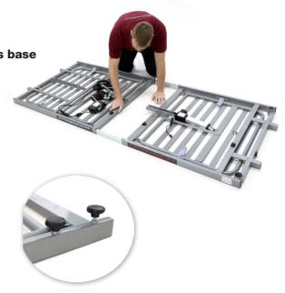
Lay the mattress base on the floor and attach the first of the bed ends to the mattress base. To do this, apply the brakes on the bed castors by pressing the brake pedal and then release the spring-loaded catches (see 6.2) at the height-adjustable head and foot end panels so the mattress base can be slotted onto the mounting lugs.
