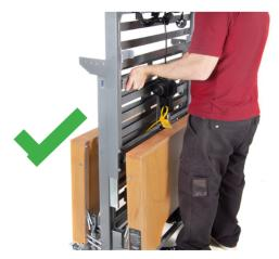
Remove the cable tie from the mains adapter and handset.
