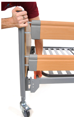
Push the end panel back towards the mattress base and place the base onto the mounting lug. Fix both the spring-loaded catches securely in place.
