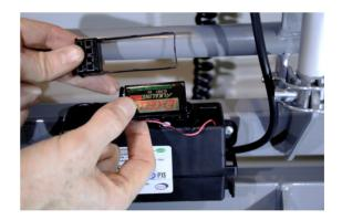
3 Reinstall the battery carrier. Be careful not to damage the wires or washer.
