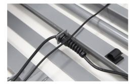
Fix the power cable to the chassis using the bracket at the head end of the bed, pull the cable taut and lock the cable grip. Secure the handset and power cable to the chassis using the cable clips attached to the platform.
