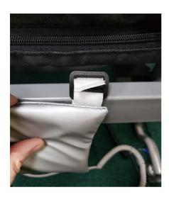
3. Position the bumper with the pad over the top of the platform and secure the strap.
