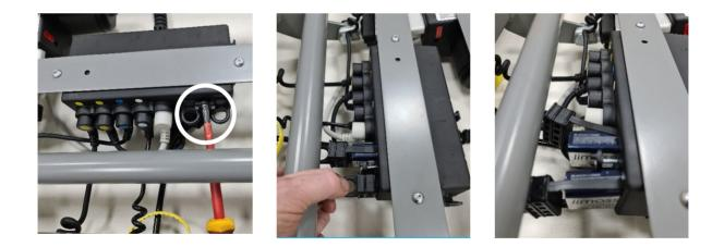
4 Reinstall the battery carrier. Be careful not to damage the wires or rubber O rings.
