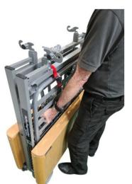
Cut the cable ties that hold the backrest in place and place the section on its side with the backrest partially raised to support the platform (take care not to open the backrest too far and allow the actuator piston to pop out, if the piston does pop out carefully re insert it).
